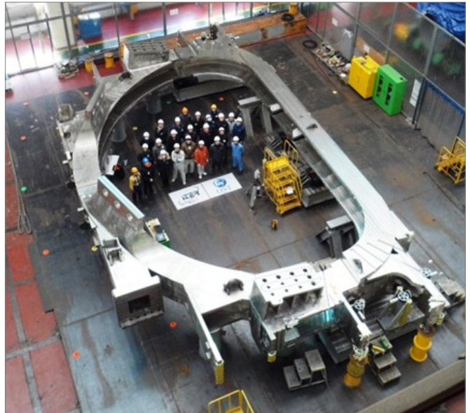
A steel case weighing over 200 tonnes that will fit over a toroidal field superconducting winding pack and provide structural support. (photo: Credit © ITER Organization)
