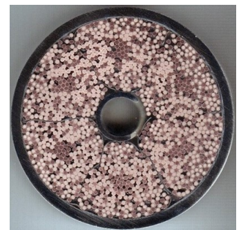
Cross-section of niobium-tin cable, showing cooling duct (photo: Credit © ITER Organization)
