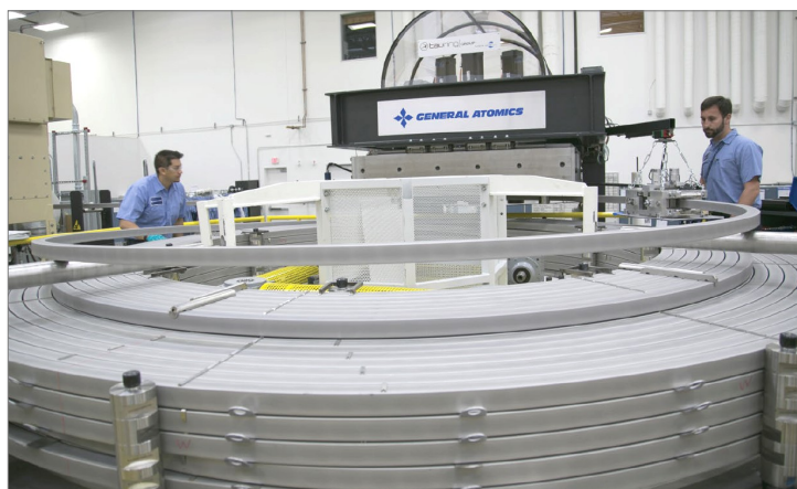
A module segment being wound using 900 m of conductor. (photo: Credit © 2018 General Atomics)
