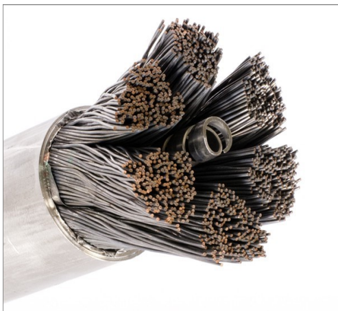
Niobium-tin superconducting cable used in the D-shaped toroidal field magnets (TF). (photo: Credit © ITER Organization)
