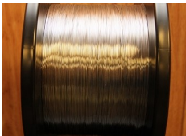
In total ITER uses 500 tonnes of Nb_3Sn (more than 100,000 km), produced by nine suppliers. (photo: Credit © Luvata)
